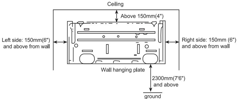
**Attention: If there are some additional function devices to install on the air conditioner, Be sure add to the installation space for the function devices.**
