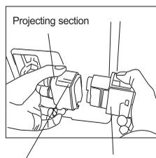
Outdoor female coupler (With movable sheath) Outdoor Valve for gas leaking
