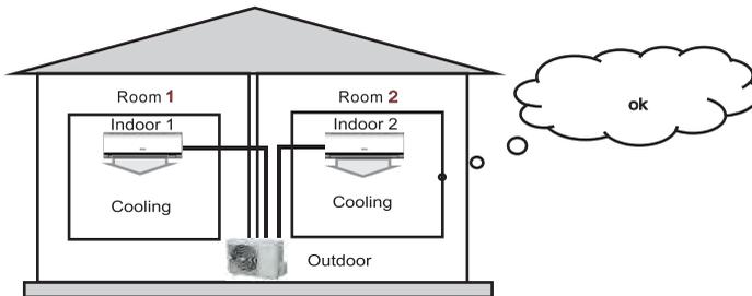
The first time the indoor is turned on, the mode of this unit is preferred. Turn off the fault indoor unit if there are mode conflict and adjust the indoor unit for the same mode. The fault will be removed automatically. Notice: the mode conflict belongs to operation fault, the mode conflict doesn't mean that this DC Inverter multi-connected has quality problems. Mode conflict chart ("√" means is normal, "x" means mode conflict).
